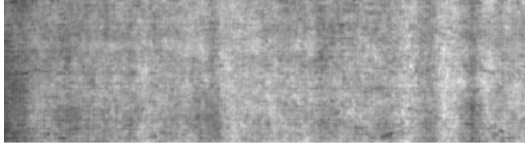
Figure 1. Example of streak distortions. The image shows an extract from a scan, the contrast has been increased dramatically. The printing direction runs horizontally, the streak distortions are thus vertical.
